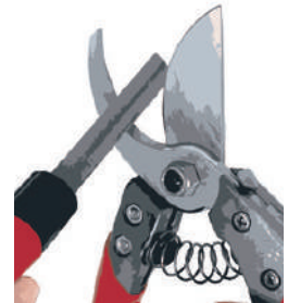
R: Receiving edge sharpening
